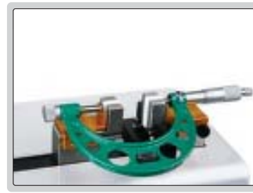
micrometer zero setting and calibration
