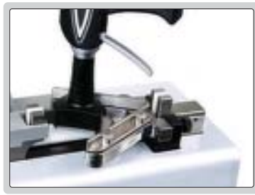
three-point internal micrometer zero setting and calibration
