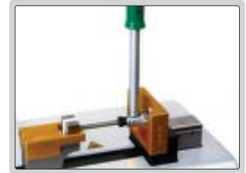
bore gauge zero setting and calibration
